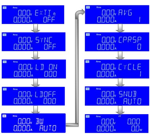
The right upper 5 digit monitor display the EXTIN and right lower monitor display OFF or ON for external input disable or enable, Default is OFF
