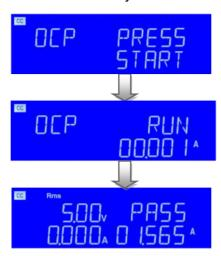
5.12.1.9. The UUT's output voltage drop-out lower than the threshold voltage (V-th Setting), and the OCP trip point is between I\_Hi and I\_Lo limitation, then Right upper 5 digits LCD display will shows "PASS", otherwise shows "FAIL".
