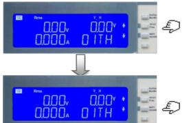
In I\_H operating modes, these can be selected in turn by pressing the "PF/CF/FREQ" key and WATT/VA/VAR Key to adjust, the setting range is 01TH ~ 50TH.
