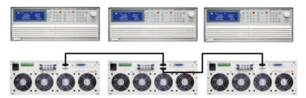
2. Boost mode is for master / slave parallel application, the setting current will be actively shared to each load, Master ammeter will show the total current that is the sum of all ammeters, Slave voltmeter will show SL1 ~ SL2, the others are unchanged.
