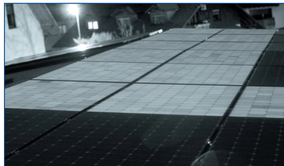
Electroluminescence image for the detection of a module strand
