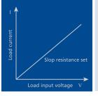
**Constant Resistant Mode** In CR mode, the module will sink a current lineary proportional to the input voltage in accor dance with the programmed resistance. Please refer to the left graph.
