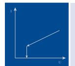
**Constant Resistance Shifting into Constant Voltage Mode** In constant resistance shifting into constant voltage mode, the measured power supply can be avoiced from current strike damage.
