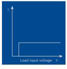
**Constant Voltage Mode** In constant current shifting into constant voltage mode, the measured power supply can be avoiced from current strike damage.
